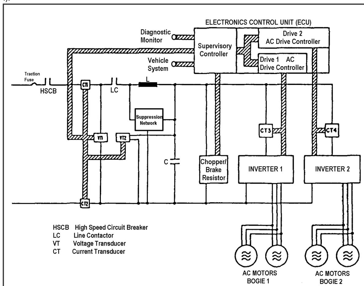
**Fig. 4 BLOCK DIAGRAM OF EMU TRACTION CONFIGURATION**
