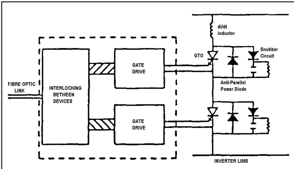
**Fig. 2 ONE ARM OF A VOLTAGE SOURCE INVERTER**
