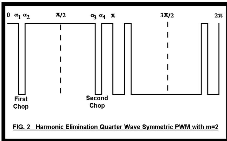
that the maximum number of harmonics that can be eliminated is  $m$ , because  $m$  independent switching angles are present in a  $0-90^\circ$  waveform section, and the rest of the cycle just reflects this section. It requires the elimination of two odd harmonics on the a.c. output of the inverter to remove just one harmonic
